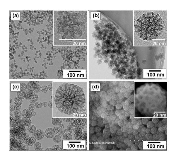
Transmission electron microscopy TEM (a, b, and c) images of prepared mesoporous SILICA NANOPARTICLES with mean outer diameter: (a) 20nm, (b) 45nm, and (c) 80nm. Scanning electron microscope SEM (d) image corresponding to (b)
